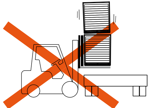
Fig.7 Packages should be unloaded one by one. Lifting two packages at once may damage a first panel in the first package.
