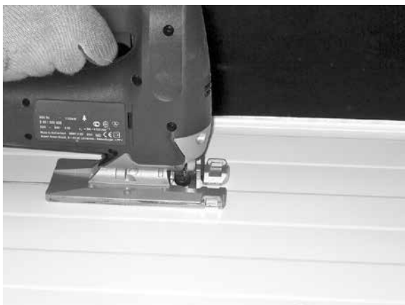
Pic. 4 and 5. Sawing machines are recommended for panel cutting.
