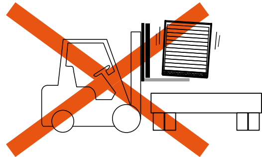
Fig.5 Too short forks may damage a package.
