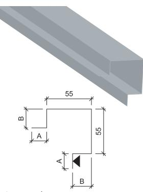
Product name Standard length Special range Blank width Weight Unit **Vertical joint flashing CA1VJ17** 3000 mm 150–4000 mm 47 mm 0,55 kg/m m
