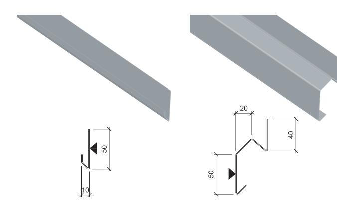
Product name Standard length Special range Blank width Weight Unit **Starting fillet CA1SF2** 3000 mm 150–3000 mm 70 mm 0,66 kg/m (steel) m
