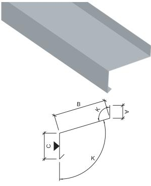
Product name Standard length Special range Blank width Minimum values Weight Unit **Plinth flashing CA1P1X** 3000 mm 150–4000 mm Depends on A, B, C measures A: 10 B: 12 C: 15 – m
