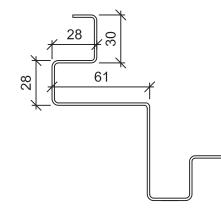
Product name Standard length Special range Blank width Weight Unit Support stud CA1RS2 3000 mm 150-4000 mm 156 mm 1,8 kg/m m
