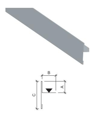
Product name Standard length Special range Blank width Minimum values Weight Unit **Cover flashing CA1C3X** 3000 mm 150–4000 mm Depends on A, B, C measures A: 20 B: 10 C: 30 m
