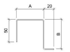
Prodcut name Standard length Special Range Blank width Weight Unit **Cover flashing CA1C16X** 3000 mm 150-3000 mm Depends on A, B measures m
