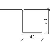
Product name Standard length Special range Blank width Weight Unit **Internal corner flashing CA1IC13** 3000 mm 150–4000 mm 178 mm 0,83 kg/m m
