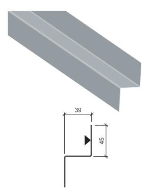
Product name Standard length Special range Blank width Weight Unit **Support flashing CA1SU2** 3000 mm 150–4000 mm 125 mm 1,2 kg/m m
